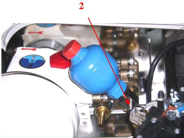
The membranes can be installed horizontally, preferably flat or on a wall support. They are mounted using 8 Parker screws in *stainless steel brackets*<sup>1</sup>. As the hose from the HP pump<sup>2</sup> vibrates, it is preferable to install the hose with an insulating tube. The HP connectors should be installed strictly in accordance with the instructions (Appendix A2). Apply a little loctite or nut seal to the two male and female cones before tightening.
