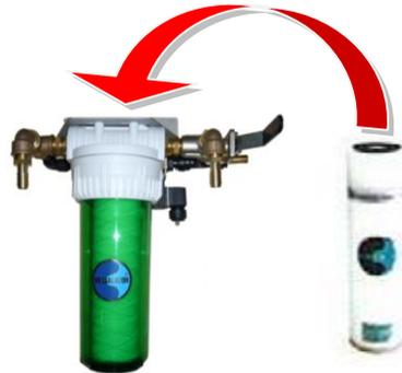
11. Set the rinsing valve to pressurized fresh water and rinse, leaving a little sterilizer in the filter.
