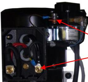
When connecting the 12 or 24V motor ensure that the polarity is correct: positive (brown wire<sup>3</sup>) on the relay and negative (green/yellow wire<sup>4</sup>) on the 12 or 24V motor. Depending on the voltage install a 12V fuse holder (supplied) or a 24V circuit breaker (supplied) on the positive cable. Ensure that the cable is of sufficient diameter: 35mm<sup>2</sup> for the 12V or 20mm<sup>2</sup> for the 24V.
