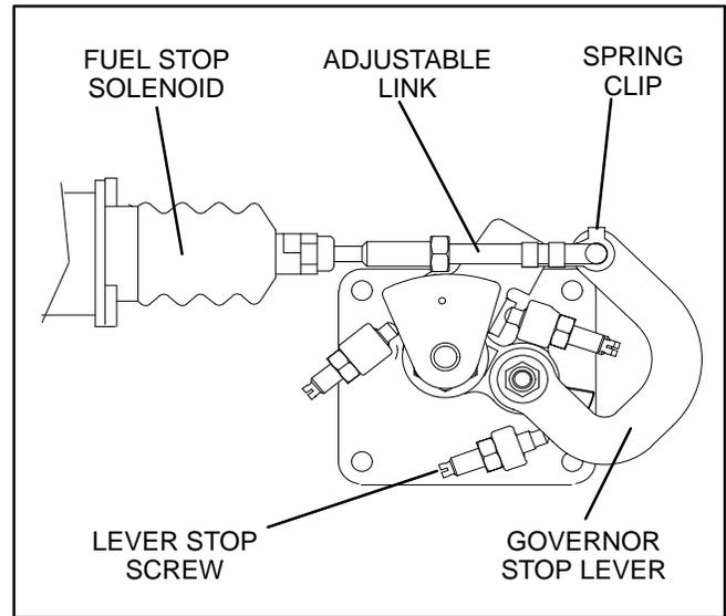
FIGURE 22. FUEL STOP ADJUSTMENT (EXCEPT MDKAL SPEC A)
