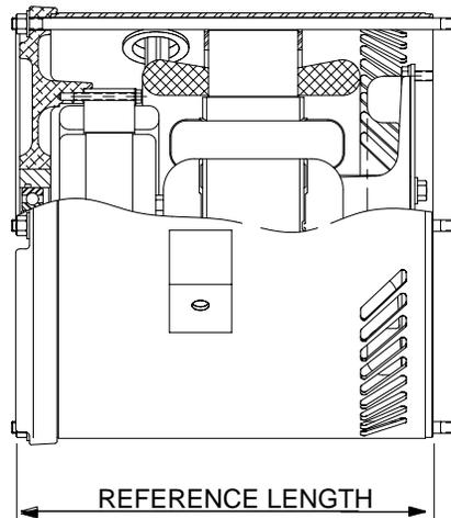
1. Measure this length to identify the generator. The corresponding rotor stack lengths are slightly greater.
