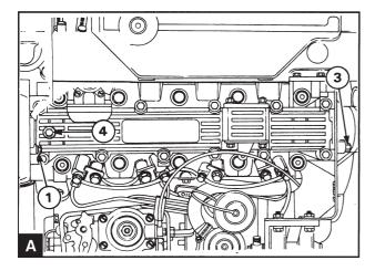
Remove the screws securing the camshaft cover front flange to the timing cover (A1).
