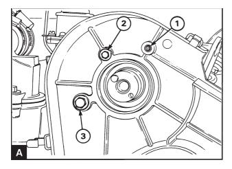
Remove the mounting screw which is installed through the camshaft cover into the timing cover (A1).
