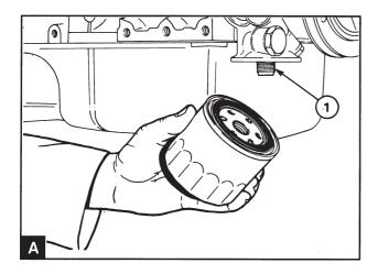
Remove the filter holder with a strap wrench or a similar tool. Ensure that the adapter (A1) remains in the filter head and discard the holder.
