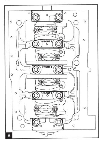
The inner main bearing caps are marked with 2, 3 and 4 and the word "FRONT" to mark the correct installation position (A). Remove the main bearing caps, the lower main bearing shells and the thrust washers. Keep the bearings with their respective caps. Press out the upper halves of the thrust washers.
