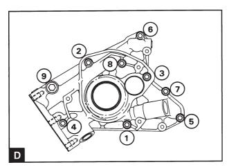
Install the pump mounting screws in position with a suitable sealing compound applied to the mounting screw which passes into the main bearing (D1). The sealing compound is already applied to new mounting screws. Tighten the screws in stages and evenly to the correct tightening torques, see Workshop Manual "Technical Data", in the correct order (D).
