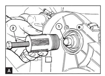
Install the plug from the tool 885026 (A1) in the front end of the camshaft. Unscrew the center screw (A2) sufficiently to ensure that it does not reach the plug and insert the main tool into the stuffing box. Turn the tool clockwise to ensure that the it is secure in the stuffing box and tighten the center screw against the plug to remove the stuffing box.
