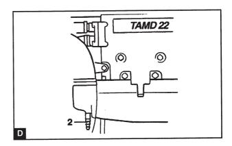
On the TAMD22 the water is drained through the cock (D2) on the charge air cooler (CAC).
