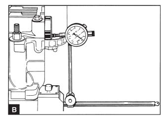
Check the camshaft axial clearance with a dial indicator (B). For tolerances see Workshop Manual "Technical data".
