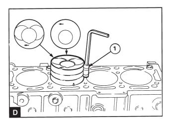
Ensure that the piston ring gaps are offset by 120° and press the rings together with a piston ring compressor (D1). Ensure that the protruberances pressed against one edge of the tool are bent downwards.
