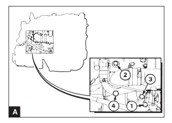
Drain the water from the heat exchanger through the cock (A4). Ensure that the drain hole is not blocked by contaminants.
