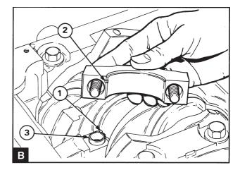
Insert the flat edge of the upper bearing shell between the main bearing journals and the side of the bearing housing which has a cut out for the lug. Slide the bearing shell into the bearing housing until the lug on the bearing shell is well inside the cut out in the bearing housing (B1).
