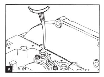
Apply sealing compound in the groove on each side of the front and rear main bearing cap (A). Apply the sealing compound until it fills the groove completely and is pressed into the column between the cap and the cylinder block. Remove the sealant from the areas around the oil pan mounting holes. Install the oil pan, operation 18A-03 within five minutes of applying the sealing compound.
