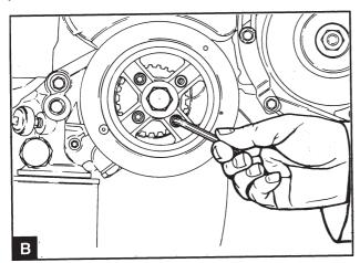
Unscrew and remove the four mounting screws (B) which secures the pulley to the belt pulley.
