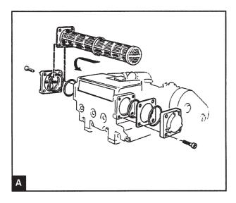
Remove the cover and press the insert out of the heat exchanger.
