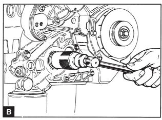
Install the adapter (A1) from the tool 885031 at the front end of the crankshaft. Slacken off the center screw so that it does not reach the adapter and insert the main tool in the sealing ring. Turn the tool clockwise to ensure that it is secure in the sealing ring and tighten the center screw against the adapter to remove the sealing ring (B). Remove the adapter.
