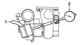
If the by-pass valve in the boost pressure control valve does not open at the correct pressure, this will affect the performance of the engine.
