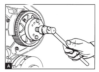
Remove the pulley with pulley puller 885027 and adapters 885029. Take care not to lose the key.
