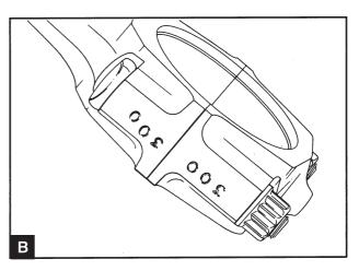
Clean the bearing shells and lubricate the bearing surfaces and big end journals. Install the upper bearing shell for the connecting rod with the locking lug well inserted in the cut out (A1). Install the connecting rod to the big end journal. Ensure that the marking on the connecting rod (B) lies in the same direction as the other connecting rods.
