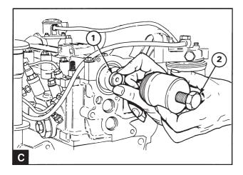
Install the plug from the tool 885019 (C1) in the rear end of the camshaft.
