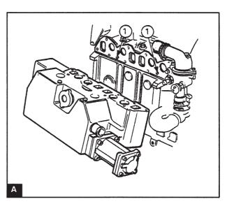
Unscrew the screws which secure the unit to the cylinder head evenly in stages in reverse order to the order shown in the illustration (B). Remove the unit (A).
