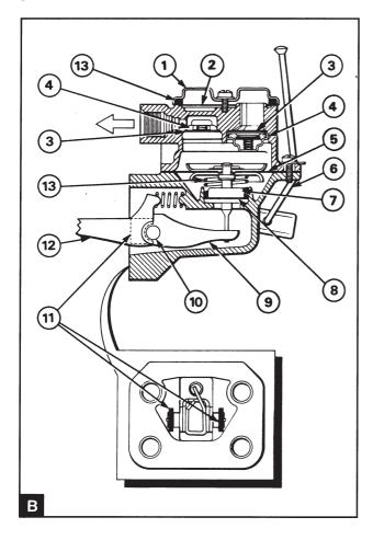
Remove the cap of the supply pump (B1) and the metal screen (B2). Remove the screws and separate the pump halves.
