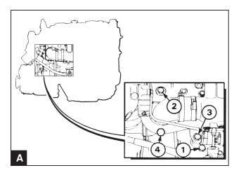
Drain the coolant by removing the plug (A1) on the starboard side of the engine block. Ensure that the drain hole is not blocked by contaminants.
