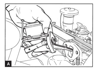
Unscrew the mounting screws and remove the supply pump (A).
