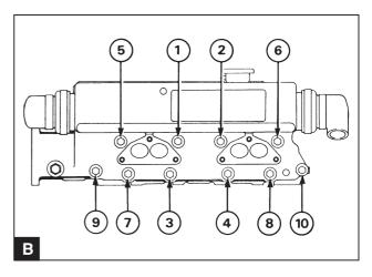
Place the unit in position on the cylinder head and install the mounting screws. Tighten the screws evenly in stages to **22 Nm** in the order illustrated (B).
