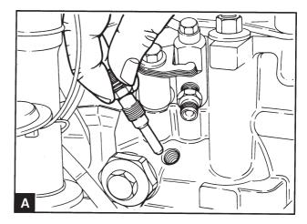
Disconnect and remove the plugs (A).
