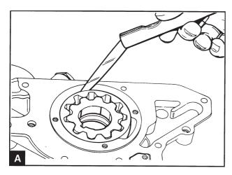
Install the rotors in the pump housing and check the outer rotor play against the housing (A).
