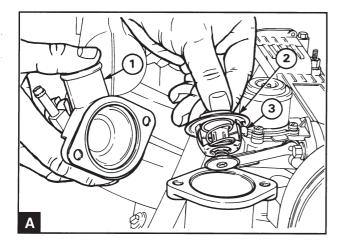
Remove the mounting screws and remove the coolant outlet connection (A1).
