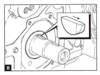
Ensure that the rear key is in position and that the bevelled end of the key is turned forwards (B). If the front key is still in position, remove it from the crankshaft.
