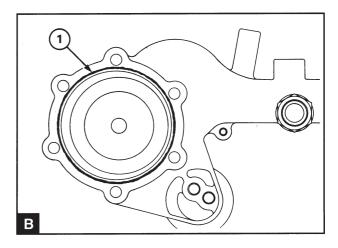
Apply a 1.0-1.5 mm continuous line of sealant on the pump mating surfaces, on the impeller side of the mounting holes (B1). If the old mounting screws are to be used, clean the threads of the screw which is to be installed at the "10 o'clock" position (A1) and apply sealant to the thread. Place the pump in position and tighten the mounting screws immediately after applying the sealant. Tighten the screws evenly in stages using the correct torque, see section 11B.
