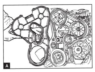
Remove the clips for the cover and remove the cap (A).
