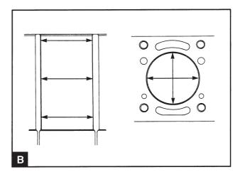
If the cylinder bores are damaged or worn more than 0.15 mm, measured in the diameter, the bore can be bored out and honed to 0.50 mm, diametrically oversize, and oversized pistons can be installed. For best results the cylinder bore should be honed with a total angle of 30° to 35° with a silicon carbide honing element which gives clean scoring. Coarse hone with a surface evenness of 1.5-2.0 mm (micrometer) and then fine hone to an mean
