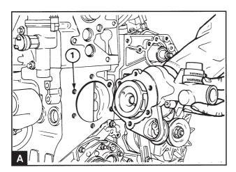
Remove the timing cover, operation 15A-08. Remove the pump mounting screws and remove the pump (A).
