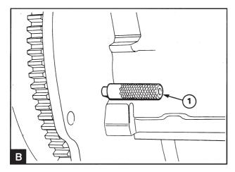
Install the adjustment drifts through the camshaft cover in the camshaft (A1) and through the flywheel cover in the flywheel (B1).
