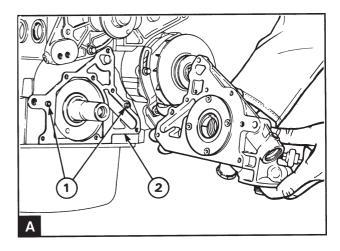
Check that the mating surfaces of the oil pump, cylinder block and main bearing cap are clean. Check that the two guide pins (A1) are in position and install a new gasket (A2).
