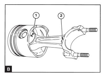
Place the connecting rod with piston upside down. The locating lug (B2) on the connecting rod must be on the same side as the arrow (B1) on the underside of the piston.
