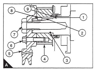
Apply a bead of Loctite 648 (A3) in a complete circle internally in the hole in the pulley (A4), 6.5 mm from the rear end panel.
