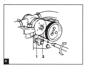
Detach the two mounting screws (A1) and (A2) and remove the belt. Remove the pump.
