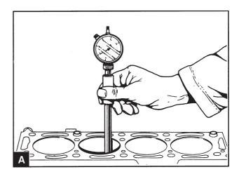
Check the cylinder bore for wear (A) and damage. The top, bottom and center of the cylinder bore should be inspected in both the vertical and lateral planes (B).
