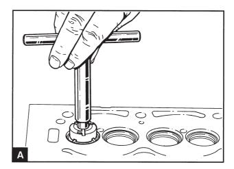
Install the mill on the locating pin with 46° side against the valve seat and install the handle (A). Do not let the mill head fall down towards the seat, this can damage the blade.
