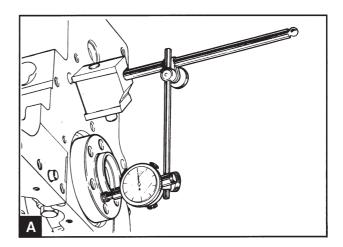
The axial play of the crankshaft is controlled by two sectioned thrust washers on each side of the central main bearing (B). The axial clearance can be checked with a feeler gauge between a thrust washer and the crankshaft. A better method is to use a dial indicator and measure axial clearance against one of the crankshaft ends (A). For the correct axial clearance, see Workshop Manual, "Technical data".
