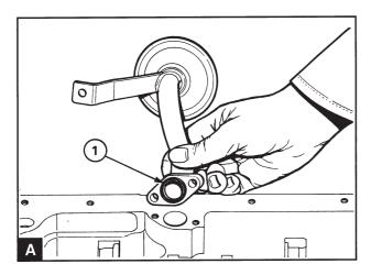
Remove the screws at the suction pipe flange and remove the suction pipe and screen. Remove the O-ring (A1). Clean the flange surface on the cylinder block and the suction pipe.
