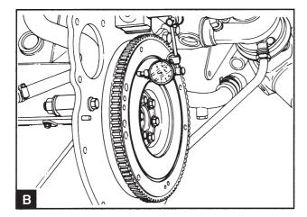
Check the axial run-out on the flywheel surface (B). The axial run-out must not be greater than 0.03 mm as a total reading on the dial indicator for every 25 mm radius of the flywheel (calculated from the center of the crankshaft to the tip of the dial indicator). During this measurement, the crankshaft must be pressed forward to prevent the axial run-out of the crankshaft from affecting the reading.
