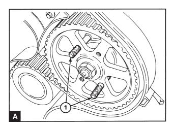
Install the two screws (M6 x 50) (A1) through the smooth holes in the fuel injection pump pulley and in the pump bracket.
