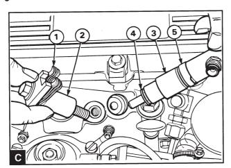
Slacken off the mounting screws for the injector holders. The spacer piece (C2) should either be 31.5mm or 7 mm long, depending on which type of injector is used. If a short spacer is used, lift the spring unit when the mounting screw is removed. This ensures that the mounting screw threads do not go in the hole in the lower spring. Remove the holder (C1) and the spacer washer. Remove the injector (C3) and the seat gasket (A4).
