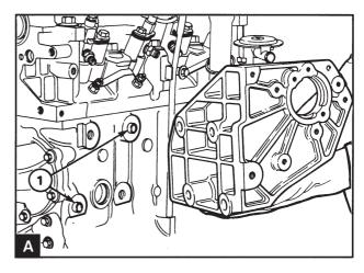
Install the fuel injection pump bracket. Check that the guide pins (A1) is correctly installed. Tighten the mounting screws to **43 Nm**.
