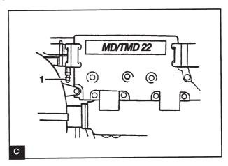
Drain the water from the heat exchanger (MD, TMD) through the cock (C1).
