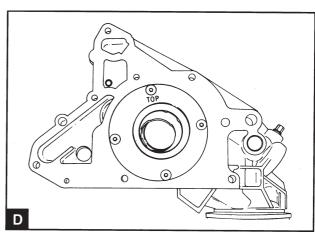
Lightly apply fresh engine oil to the rotors and insert them in the pump. The inner rotor has a lug in one end and this tap must be turned towards the sealing ring housing. Install the back plate with the word "TOP" turned from the pump housing straight edge (D). Install and tighten the screws for the back plate to **4 Nm**.
