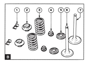
Take the load off the valve spring tensioner and remove the valve spring washer (B2), valve spring (B3), valve stem seal (B4) and the spring seat washer (B5). Remove the exhaust valve (B6) or the inlet valve (B7).
