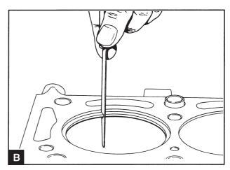
Check that all the soot has been removed from the upper section of the cylinder bore. Install the piston rings in the upper section of the cylinder bore and measure the ring gap with a feeler gauge (B). The expander ring must be installed on the oil scraper ring when the ring gap is measured. The ring gap for the new components is given in the Workshop manual "Technical data".
