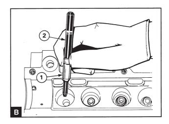
Install the guide B1 on the thin end of the tool 885021 (B2) with the bevel turned to the thin end of the tool (B). Insert the bevelled end of the guide into position in the cylinder head and press in the guide until the tool end comes into contact with the flat plate. Check that the guide protrudes 10 mm above the mating surface for the valve spring.
