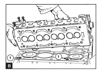
Unscrew the screws for the cylinder head evenly in reverse order compared to the illustration 12A.09/A. Remove the screws and dismantle the cylinder head (B), ensure that the camshaft does not come into contact with the timing cover. Place the cylinder head on even surface that will not damage the cylinder head surface.
