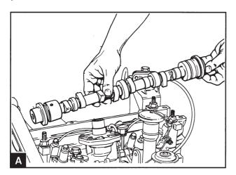
Remove the camshaft (A) and remove the camshaft sealing rings.
