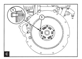
Install the elastic disc for the reverse gear (C). Apply Locktite 243 on the threads of the mounting screws for the disc. Ensure that the small guide section of each mounting screw goes into the flywheel (C1). Tighten the mounting screws evenly in stages to 9 Nm. Do not start the engine until the locking fluid has hardened.
