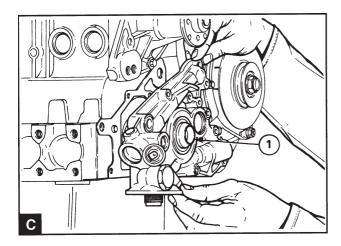
Clean the crankshaft and the protective socket 885032-3 and lightly lubricate with fresh engine oil. Install the protective socket (C1) on the crankshaft.
