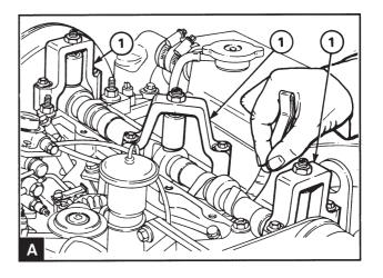
Install the camshaft mountings 885024 (A1) to hold the camshaft and mount the mountings with the relevant mounting screws for the cover. It is vital to move the rear camshaft stuffing box on the camshaft to secure sufficient clearance between the rear mounting and the stuffing box. Ensure that the sprung pads are correctly installed on the camshaft bearing journals and tighten the mounting screws for the mountings evenly.
