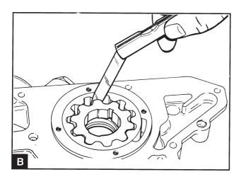
Check the inner rotor clearance against the outer rotor (B).
