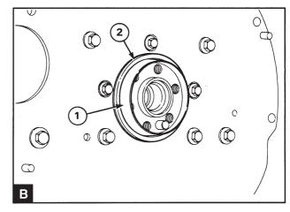
Clean and lubricate the protective socket 885030 (B1) and install it on the end of the crankshaft flange.
