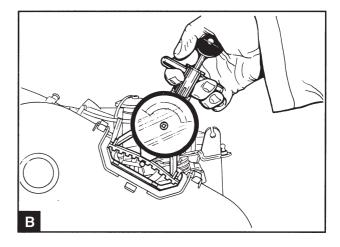
Press the ball end of the belt tension gauge and install the gauge over the belt. Ensure that the gauge foot is located under the belt and between two teeth (B). Slowly release the ball end and read off the gauge. Turn the crankshaft slightly in each direction until a stable read off is obtained. The correct value for a new belt is 425-465 N and for a used belt 340-370 N. If the tension of a used belt has fallen to 270 N or below, adjust the belt tension to 340-370 N, operation 15A-03.
