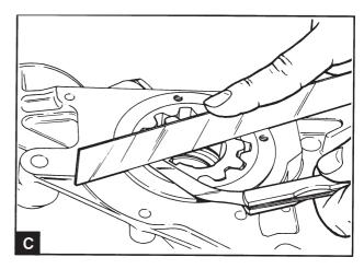
If the sealing ring needs changing, remove the rotors and press the sealing ring out of the housing. The pump is easier to install on the engine with the sealing ring uninstalled and the sealing ring can be installed on the installed pump, see operation 14A-02.
