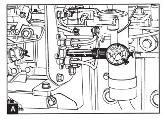
Remove the plug and the washer from the center of the fuel injection pump rear plate and install the gauge. Set the gauge so that it reads approximately 3.0 mm. Ensure that there is sufficient play between the gauge and the oil filler pipe, to allow for any radial movement in the pump.
