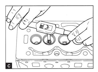
Ream the hole for the new guide using reamer 885022 (C).
