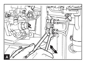
Remove all the necessary pipes from the pump. Use a wrench as a counterhold at the pump outlets side (A) to prevent the joint moving when the nuts for the delivery lines are slackened off.
