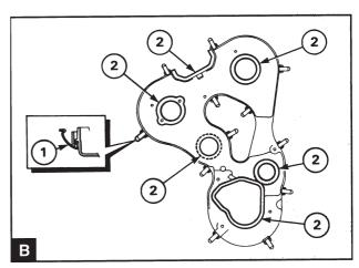
Check the timing cover for cracks and damage and replace it if required. Check that all the clips are correctly installed in the timing cover (B1).
