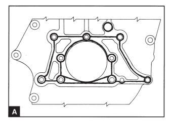
Apply a continuous 1.5 mm line of sealant on the front surface of the cover, as shown in illustration A. This operation is not necessary if a separate housing is installed for the stuffing box.
