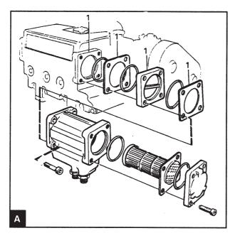
Make a mark on the flanges (A1) and the coolant tank, so that the flanges can be reinstalled in the same position.
