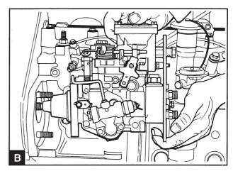
Remove the locknuts and remove the pump (B) – ensure that the key does not fall out of the drive shaft.
