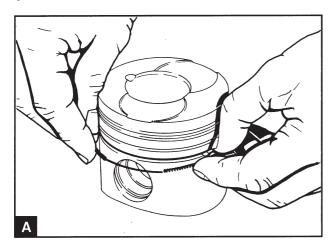
Insert the expander ring for the oil scraper ring in the lower piston ring groove with the catch through both end of the rings (A). Install the oil scraper ring over the spring (B). Ensure that the ring gap is located with a 180° offset to the catch.
