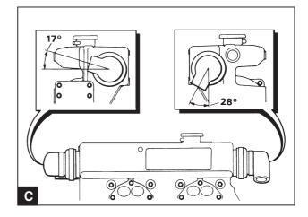
Install the second rubber end. Check that the pipe connectors of the rubber ends are in the correct position and tighten the clamps. Place the rubber ends in the positions shown in C if the assembly has be removed from the engine.
