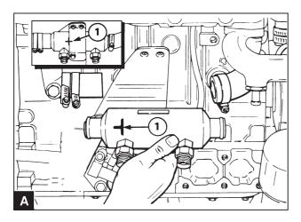
Make a mark with a felt-tip pen on the oil cooler housing and on the clamp (A1) in order to be able to reinstall the oil cooler in the same position.
