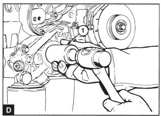
Install protective socket 885032 (C1) on the crankshaft. Lubricate the new sealing ring with fresh engine oil. Insert the sealing ring in position over the protective socket with the seal lip turned towards the engine. Remove the protective sleeve. Use installation tool 885033 (D1) and a hammer with a soft face to drive the sealing ring into the correct position. The correct position for the sealing ring is when the sealing ring front surface is 0.5 mm inside the housing.
