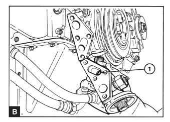
Clean the sealing surfaces on the oil filter adapter and the oil pump.
