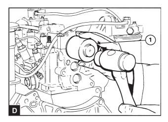
Ensure that the stuffing box and the camshaft are clean and undamaged. Lubricate the new stuffing box with fresh engine oil and insert it into position with the seal lip inwards. Use installation tool 885020 (D1) and a hammer with a soft face to drive the stuffing box into the correct position.
