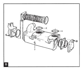
Remove the charge air cooler assembly from the heat exchanger. Remove the cover and the plugs (B1 and B2). Press the insert out of the heat exchanger.
