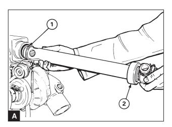
Press out the insert in whichever direction. Ensure that the sleeve (A1) also comes out of the heat exchanger.
