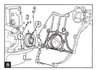
Check that the guide pins (B1) are correctly installed. Check that the outer diameter of the crankshaft flange is clean. Install the protective sleeve for the stuffing box (B2) in position on the crankshaft flange. Lightly lubricate the outer diameter of the crankshaft flange and the protective sleeve with fresh engine oil.
