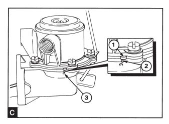
Press the rocker arm upwards in the diaphragm until the diaphragm lies at the level of the pump housing flange. Install the upper half of the pump housing in position with the marks on the flanges lined up. Keep pressure on the rocker arm and install the spring washers and screws. Remove the pressure from the rocker arm and tighten the screws evenly. After installation the edge of the membrane should lie along at the level of the edge of the pump housing.
