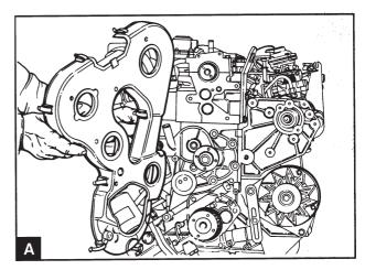
Unscrew the screws securing the timing cover to the cylinder head, the cylinder block, the fuel injection pump bracket and the oil pump. Remove the timing cover (A).
