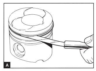
Install the new piston rings in the piston ring groove and check the ring groove wear using the feeler gauge (A). Compare the piston ring play in the groove to the values that apply to new components in the Workshop Manual "Technical Data". Replace the cylinder if necessary.
