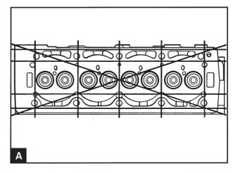
Use a straight edged ruler and a feeler gauge to check the latitudinal, longitudinal and diagonal flatness of the bottom surface of the cylinder head (A). If deformation is greater than 0.10 mm the bottom surface can be machined. Remove the minimum amount of material and check that the cylinder head height will not be less than 119.85 mm after the cylinder head has been treated.
