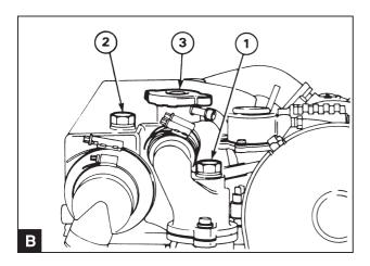
Remove the bleed plug from the hot water connection (B1) or the plug (B2) on the heat exchanger.
