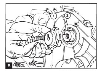
Remove the mounting screws for the pulley and remove the pulley. Remove the pulley hub (B1) and the guide pin (B2).
