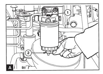
Carefully clean the outside of the fuel filter unit. Slacken off the bleed screw (A1) located above the filter, two or three turns. Slacken off the drain arrangement (A2) at the bottom of the holder and drain the fuel into a suitable container. 2
