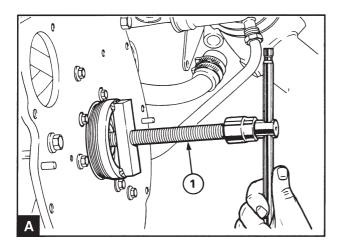
Slacken off the screw (A1) in the puller tool so that it does not reach the crankshaft. Insert the tool in the sealing ring and turn it clockwise so that it fastens in the sealing ring. Use an adjustable spanner to turn the tool body so that it fastens securely in the sealing ring. Tighten the screw against the rear end of the crankshaft in order to remove the sealing ring.
