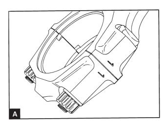
Check that all the connecting rods and the caps are marked with the correct cylinder number (A). If they are not marked, mark them from 1 to 4 with the number 1 at the timing belt cover end.
