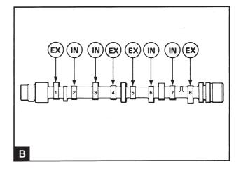
The valve clearance is measured between the camshaft and the upper side of the valve lifter (A). With a cold engine the correct valve clearance 0.25-0.35 mm for the inlet valves and 0.35 –0.45 mm for the exhaust valves. See B for the position for the inlet and exhaust cams.
