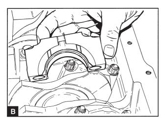
Install the lower thrust washer halves in the main bearings with the lugs in their respective cut outs. Check that the lubrication grooves in the thrust washers are turned away from the bearing cap (B).
