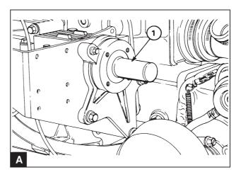
Position alignment tool 885038 (A1) with the narrow diameter in the camshaft and the wider diameter in the adapter plate. Tighten the mounting screws evenly in stages and remove the alignment tool.
