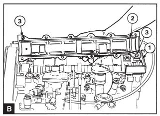
Remove the engine lifting brackets. If nothing is driven from the rear end of the camshaft, remove the rear cover and install the camshaft lock 885025 (B1). This ensures that the camshaft does not tilt when the camshaft cover is removed.
