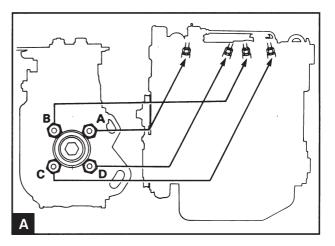
Install the delivery pipes to the pump. Use a wrench to prevent the output terminals on the fuel pump (FP) from moving when the delivery lines are installed. The connections to the pump are as displayed in illustration A. Do not tighten the connector to the injectors until the system has been bled.
