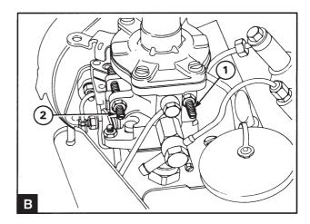
Run the engine to operating temperature and check the idling speed. If required adjustment can be carried out using the inner adjustment screw (B1). Slacken off the locknut and turn the screw clockwise to increase and counter-clockwise to decrease the engine speed (RPM). Tighten the locknut when the engine speed (RPM) is correct.
