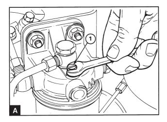
Slacken off the bleed screw (A1) located above the fuel filter, two or three turns.
