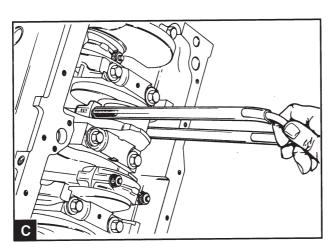
Install rubber or plastic protective tubes on the connecting rod screws (B1). Slide the piston and the connecting rod upwards in the cylinder bore A suitable tool for this job can be made from a (U) shaped pipe and two pieces of plastic hose (C).
