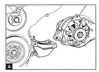
Remove the adjuster link from the generator and remove the pivot shaft. Note the position of the washer to ensure that it is correctly installed. Remove the generator (A).
