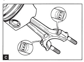
Check the condition of the connecting rod screws. If the thread is sealed or if there are signs of stretching, the screw must be removed from the connecting rod and replaced. The new screw must be installed with the locating arrows (or recognition marks) on the screw head turned to the outside of the connecting rod big end (C). Ensure that the screw head has good contact with the connecting rod.
