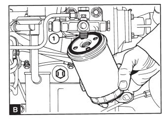
Use a strap wrench or similar to remove the filter (B).
