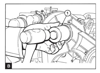
Ensure that the stuffing box and the camshaft are clean and undamaged. Lubricate the new stuffing box with fresh engine oil and insert it into position with the seal lip inwards. Use installation tool 885026 (B1) and a hammer with a soft face to drive the stuffing box into the correct position.
