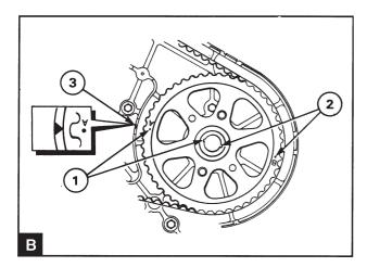
Install the pulley in position on the shaft with the correct keygroove in contact with the key. There are two keygrooves and two marked teeth, "A" and "B", on the pulley. On engines types MD22 and MD22L use the keygroove lying on the same side as the tooth marked "A". On engines types TMD22 and TAMD22 use the keygroove lying on the same side as the tooth marked "B". Ensure that the marking on the pulley is turned to the front end of the engine.
