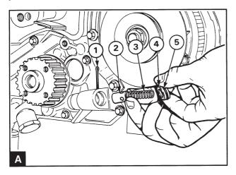
Bend the shafts of the split pin together (A1). Press the end plug (A4) and remove the split pin from the pump housing.
