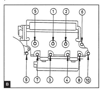
Place the unit in position on the cylinder head and install the mounting screws. Tighten the screws evenly in stages to **22 Nm** in the order illustrated in B.
