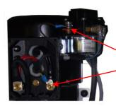
When connecting the 12 or 24V motor ensure that the polarity is correct: positive (brown wire<sup>3</sup>) on the relay and negative (green/yellow wire<sup>4</sup>) on the 12 or 24V motor. Depending on the voltage install a 12V fuse holder (supplied) or a 24V circuit breaker (supplied) on the positive cable. Ensure that the cable is of sufficient diameter: 35mm² for the 12V or 20mm² for the 24V.
