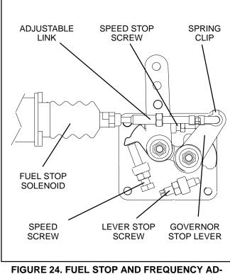
GURE 24. FUEL STOP AND FREQUENCY AD JUSTMENTS (MDKAL SPEC A)
