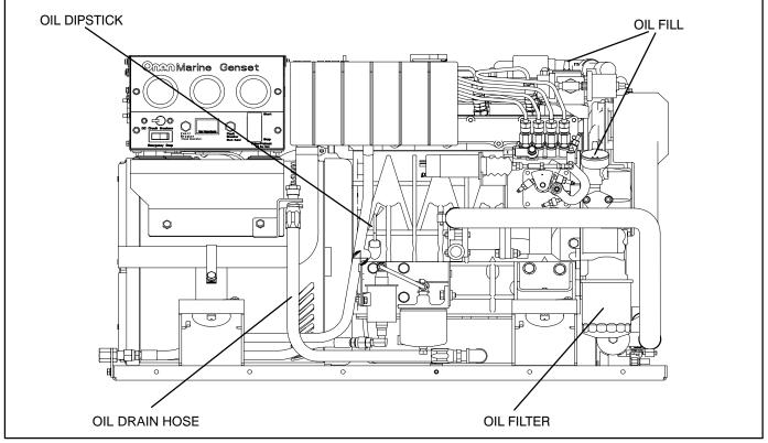
FIGURE 4. OIL CHECK, FILL, DRAIN AND FILTER
