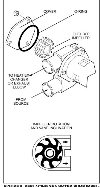
FIGURE 9. REPLACING SEA WATER PUMP IMPEL-LER
