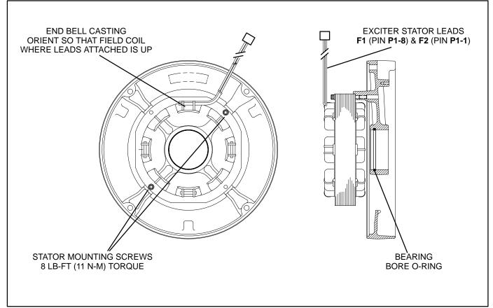
FIGURE 18. EXCITER STATOR AND END BELL
