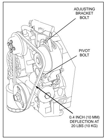
FIGURE 6. ADJUSTING V-BELT TENSION
