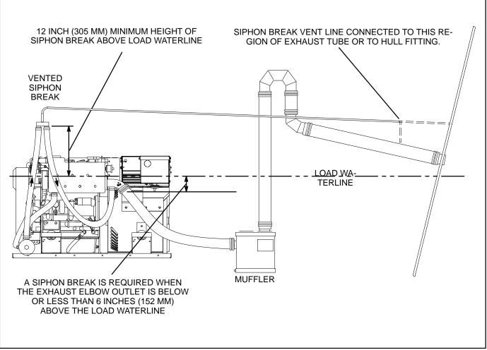
FIGURE 8. TYPICAL INSTALLATION OF A VENT-TYPE SIPHON BREAK AND WET EXHAUST SYSTEM
