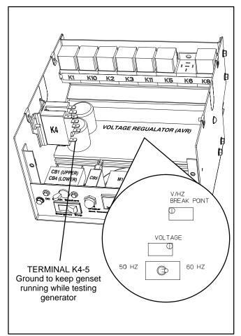
FIGURE 15. VOLTAGE REGULATOR (AVR)
