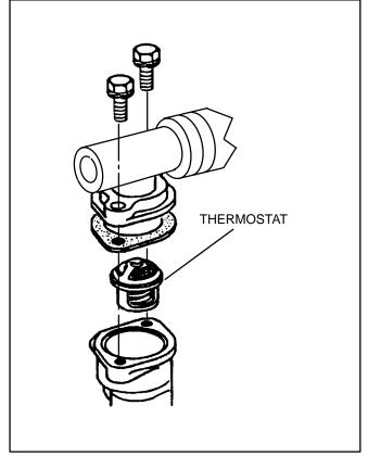
FIGURE 7. REPLACING THERMOSTAT
