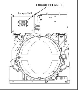
FIGURE 3. GENSET MOUNTED LINE CIRCUIT BREAKERS
