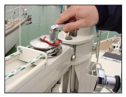
Picture 20 – Release of the electric clew's motor
