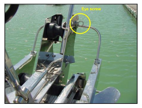
Picture 87 – Fitting for 2 anchors
