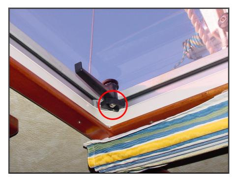
Picture 97 – Blocking up a deck hatch
