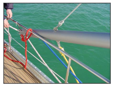
Picture 30 – Attachment of the lines on the pole and way of jib's sheet
