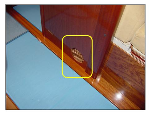
Picture 76 – Clothes' washer / dryer intake
