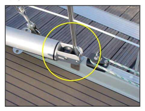
Backwards, the pole's block is set on the base of the stanchion.
