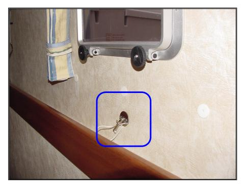
Picture 53 – Locking the opening of the engine room's cover
