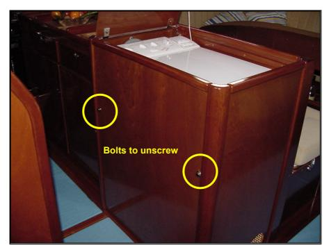
Picture 102 - Removal of the clothes washer / dryer
