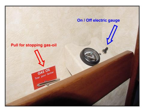
Picture 50 – Gas-oil electric gauge and lever for stopping gas-oil delivery from the passageway
