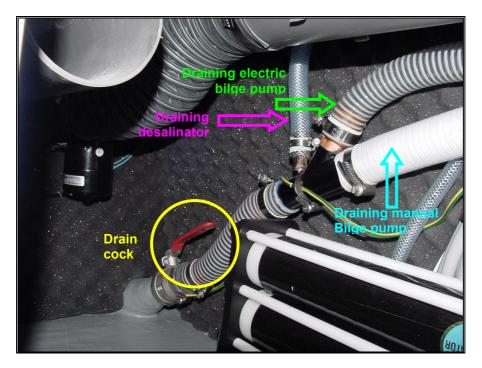
Picture 59 – Wasted water drain cock (photographed open)
