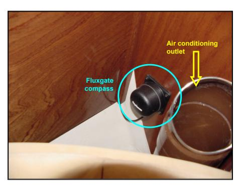
Picture 94 – Fluxgate compass
