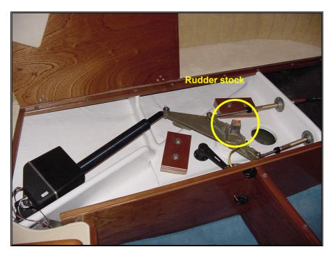
Picture 10 – Rudder stock and automatic pilot linear driving unit
