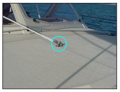
Picture 39 – Setting the tack on the mizzen ballooner
