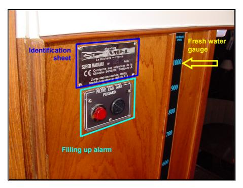
Picture 57 – Seawater and sump alarm
