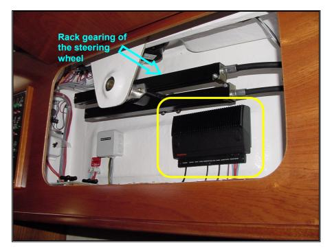
Picture 93 – Automatic pilot's calculator of the steering wheel
