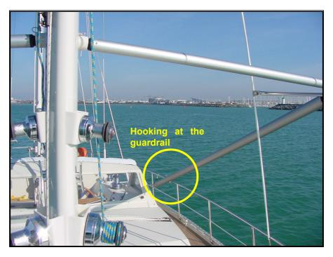
Picture 29 – Pole hooked to the guard-rail
