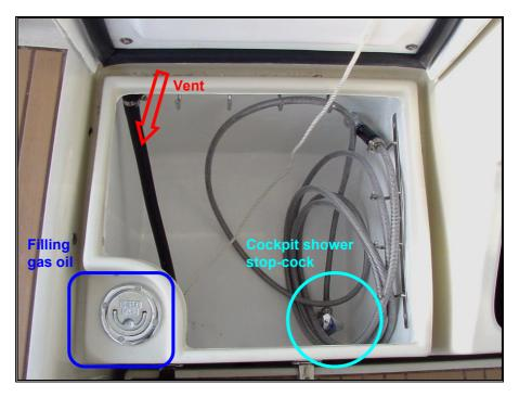
Picture 47 – Starboard cockpit locker
