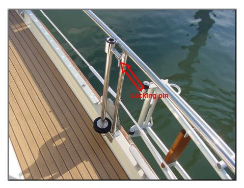
Picture 24 – AMEL's jib sheet traveller remote control
