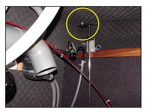
Picture 51 – Stopping gas-oil delivery from the engine room
