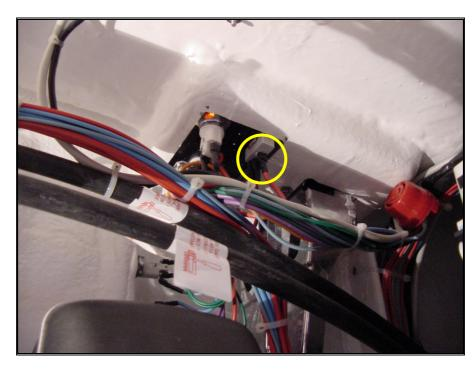
Picture 2 – Plug to disconnect when the boat is out of the water
