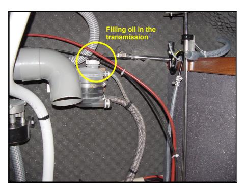
Picture 5 – Transmission oil tank
