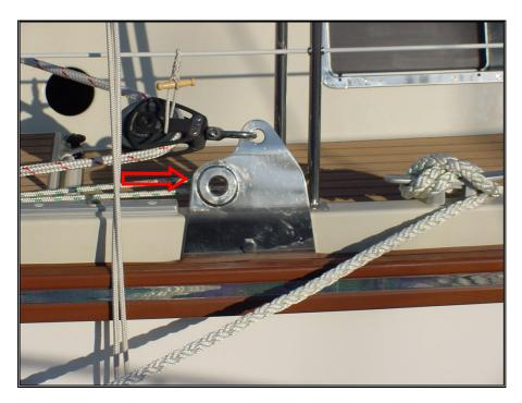
Picture 100 – Aft lift U-bolt
