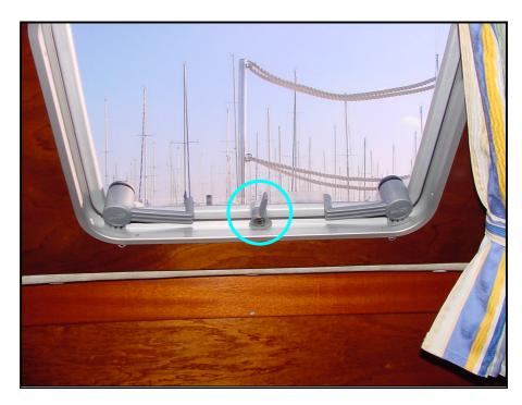
Picture 98 – Blocking up the aft cabin hatch
