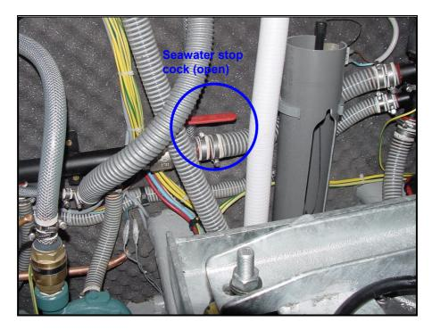
*Picture* 58 – Seawater stop cock (other devices as main engine and generator)
