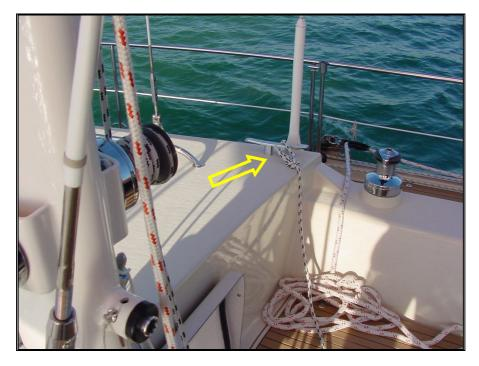
Picture 41 – Halyard secured before hoisting
