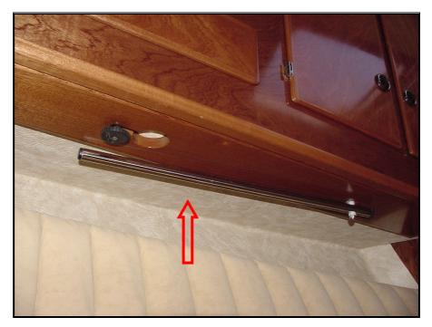
Picture 78 – Storage of the forward cabin's wooden lee board
