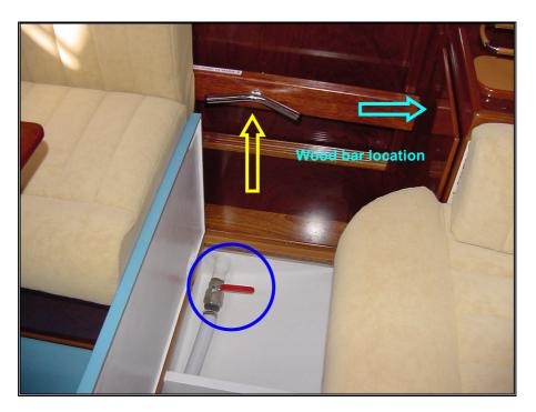
Picture 43 – Wood bar settled and forward compartment seacock (photographed closed)
