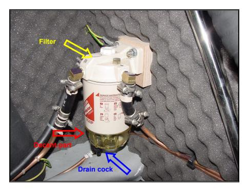
The RACOR-filter delivers gas-oil to the main engine and the generator.
