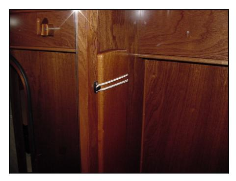
Picture 82 – Storage of the aft cabin's wooden lee board
