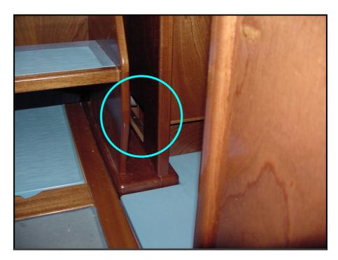
Picture 75 – Refrigerator's air intake
