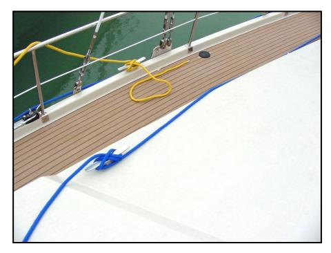
send the pole running up the blue rope, and take it on the cleat, \_
