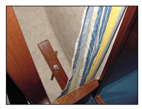
Picture 45 – Storage of the aft wood bar
