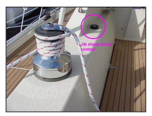
Picture 11 – Jib sheet electric winch
