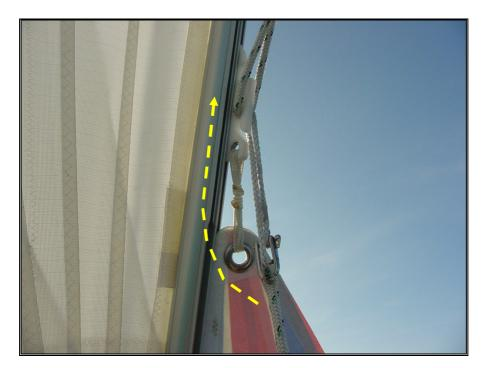
Picture 35 – Hook engaged in the jib foil
