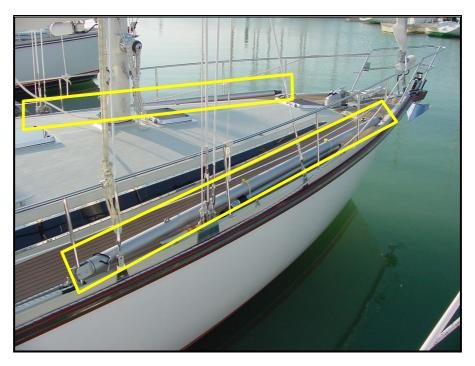
*Picture 26 – Pole and jockey pole* Forward, the pole is plugged onto a pin (part of the stanchion).
