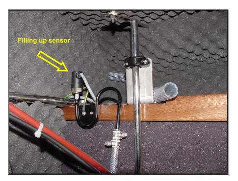
Picture 56 – Blockage sensor of the seawater filter
