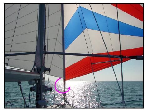
Picture 36 – Furling the jib and the ballooner together
