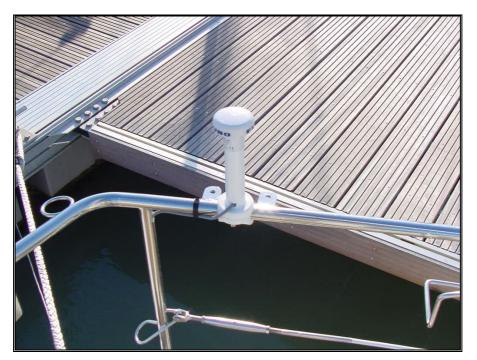
The GPS' antenna is mounted on portside aft of the stainless steel guard-rail.
