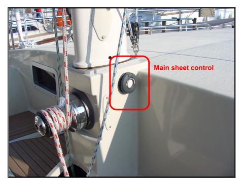
Picture 12 – Main sheet electric winch
