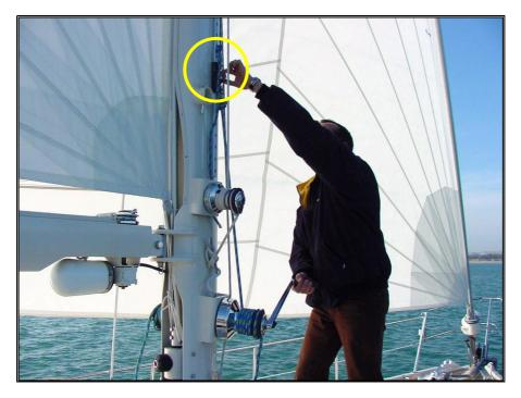
Picture 16 – Tightening the mainsail halyard
