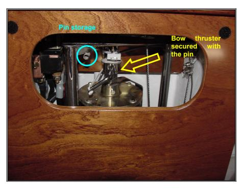
Picture 1 – Bow thruster electric motor, jack and pin
