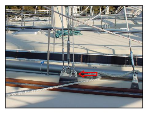
Picture 99 – Forward lift U-bolt
