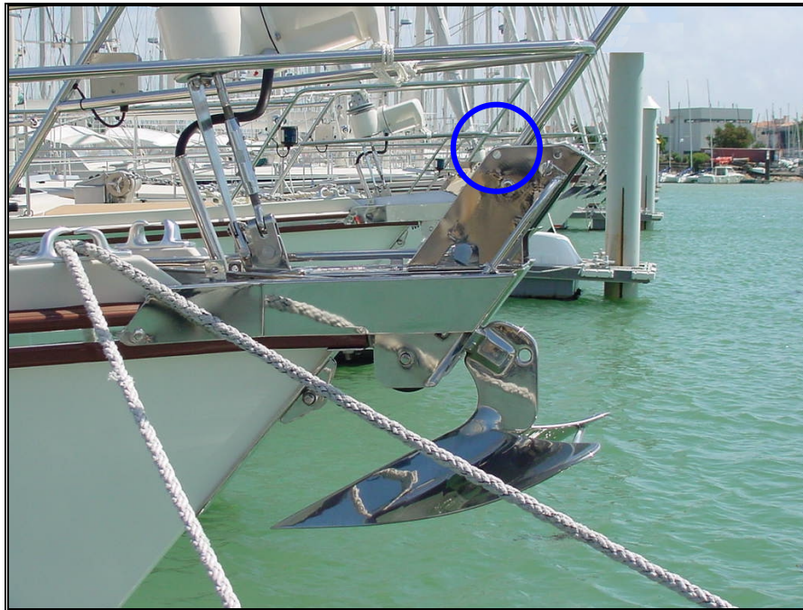
Picture 34 – Tack point on the anchor fairlead
