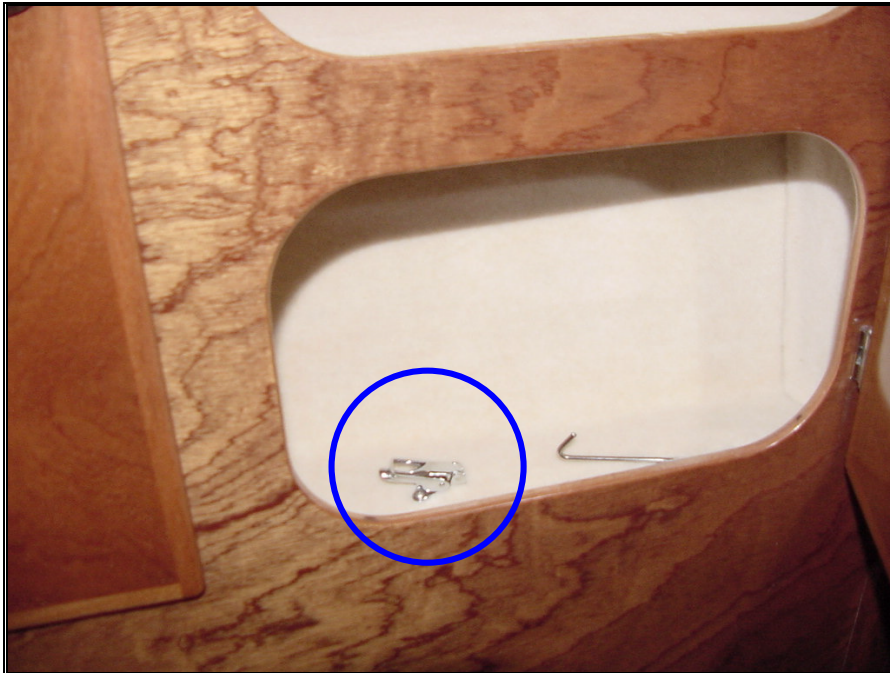
Picture 21 – Closing the fresh air ventilation outlet from the saloon
